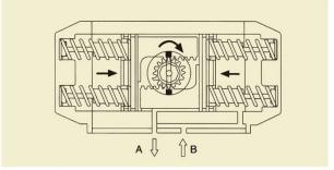
In the event of loss air pressure or power, the stored energy in the springs forces the pistons inwards, causing the pinion turns clockwise while air is being exhausted from Port A, and air to Port B can accelerate closing the valve.
