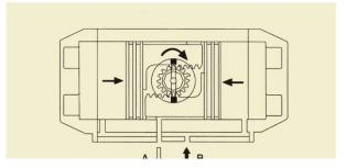
Air into Port B forces the pistons inwards, causing the pinion to turn clockwise while the air is being exhausted from Port A.
