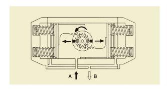
Air into Port A forces the pistons outwards, causing the springs to compress, the pinion turns counterclockwise while air is being exhausted from Port B.
