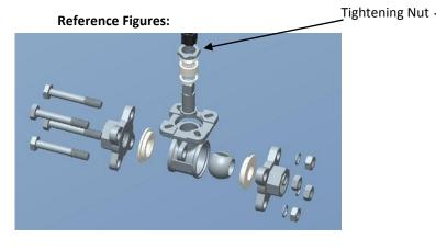
**Figure 1:** Exploded view of valve body with tightening nut indicated.
